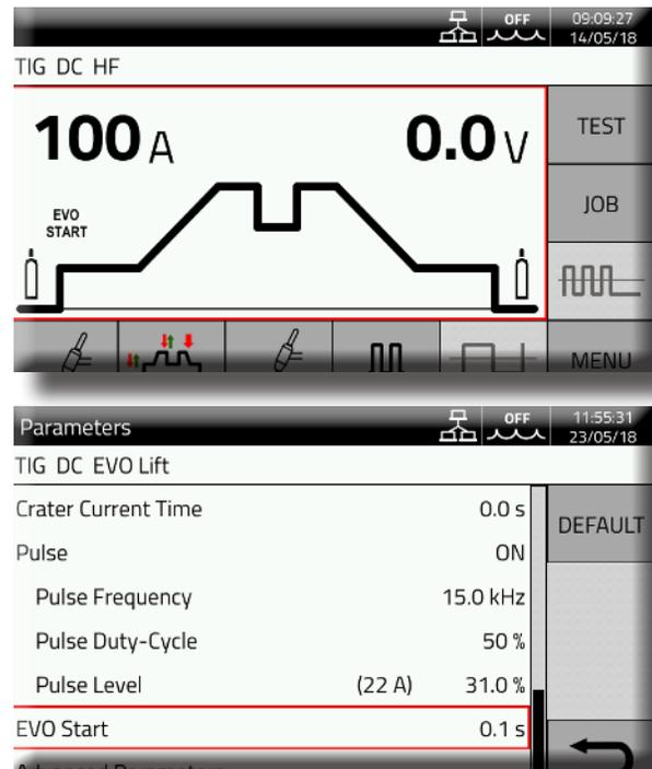
**WIN TIG DC 500 T** is a three-phase power source with inverter technology for TIG and electrode (MMA) DC welding, with built-in HF ignition. Comes with cooling unit and trolley for transportation of the power source. Can be connected to the wireless auto darkening filter (art. 434-optional) for protection mask.
